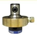
Important: coolant flow must be started prior to rotating the spindle to avoid damage of the Orings
